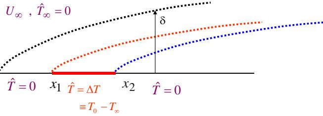
$$-k \left( \frac{\partial \hat{T}}{\partial y} \right)_{y=0} = \frac{d}{dx} \int_0^{\delta_T} \rho c_p u \hat{T} dy \quad \text{where } \hat{T} \equiv T - T_\infty$$
