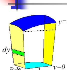
pressures forces =  $\left( \int_0^Y p R d\phi dy \right)$
