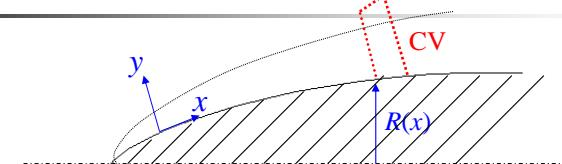
$$-\tau_0 = \rho_0 v_0 U_\infty - \rho_\infty U_\infty \frac{dU_\infty}{dx} - \frac{U_\infty}{R} \frac{d}{dx} \left( R \int_0^y \rho u dy \right) + \frac{1}{R} \frac{d}{dx} \left( R \int_0^y \rho u^2 dy \right)$$
